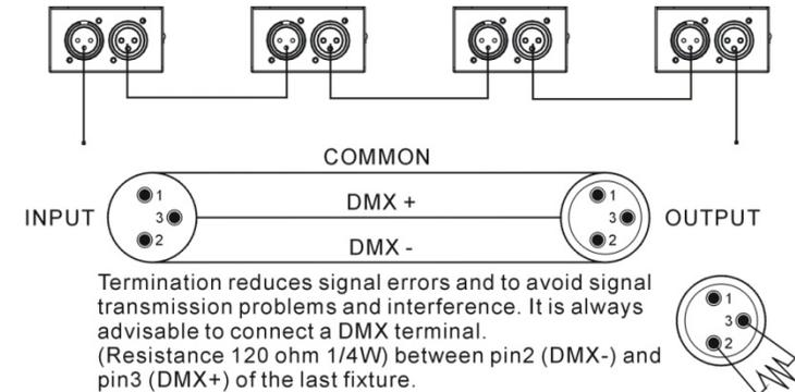
1. If you using a controller with 5 pins DMX output, you need to use a 5 to 3 pin adapter-cable.
