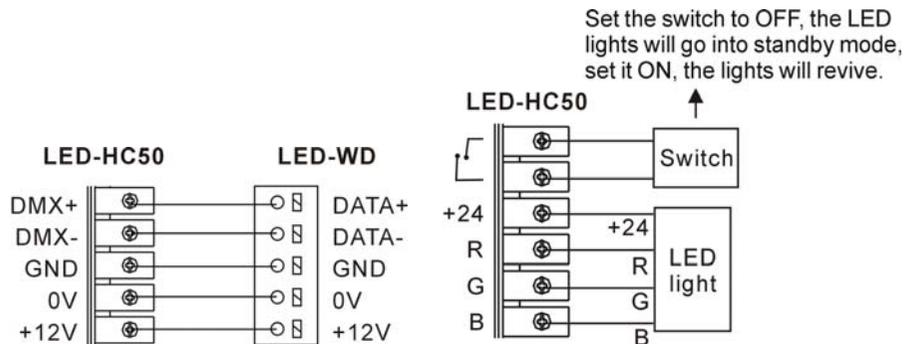
**CAUTIONS :** the LED controller total output power consumption is 50 watt.
